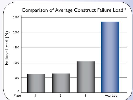
**Summary:** Biomechanical tests show that the Acu-Loc plate can withstand a force far beyond the loads that are seen in the radius during patient rehabilitation.
